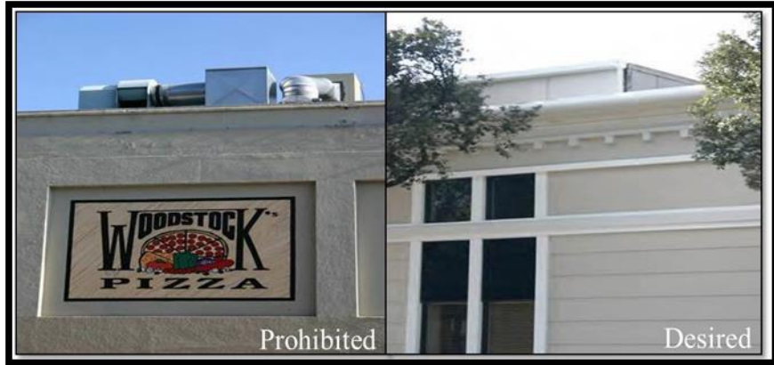
Figure 15.3-22. Rooftop Utilities Screening
